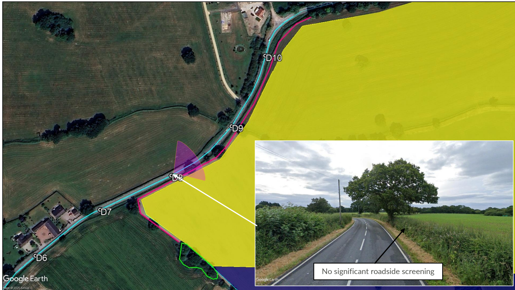
Figure 13 Reflective panel area and proposed screening for road receptors D6 to D10
