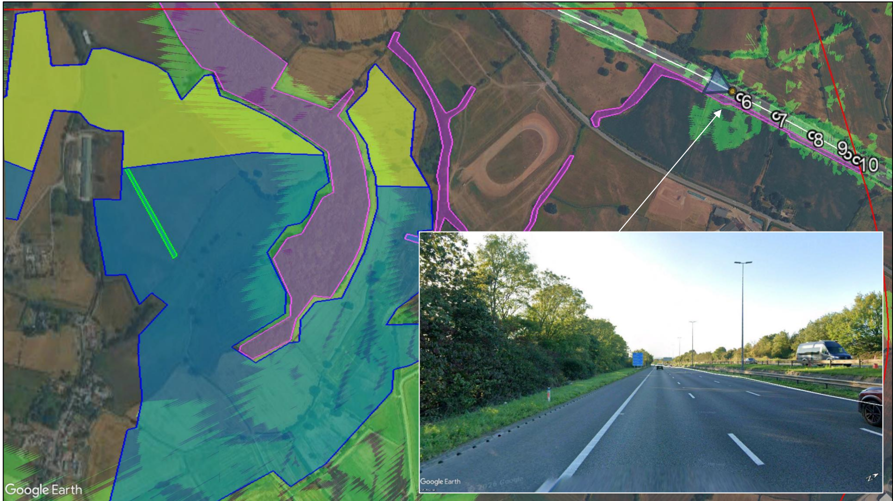
Figure 21 Screening relevant to road receptors 6 to 10, with representative ZTV viewshed from receptor 7
