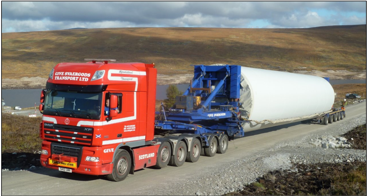
Figure 3: Base Tower Trailer
